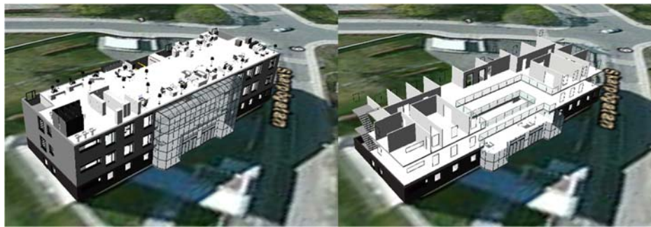
Fig. 6. Left: Third floor exclusive view of property elements (furniture) Right: Second and Third floor combined view of stairs, inner walls, doors and windows
