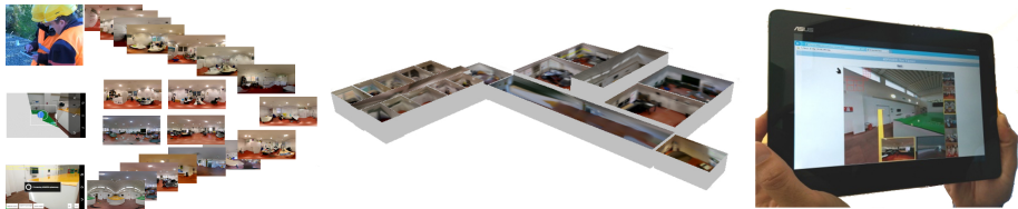
Fig. 1. Our method at a glance: from a set of panoramic photos (left) our system computes a textured 3D model of the indoor boundaries (center) which can be explored with a low-degree-of-freedom web application (right).
